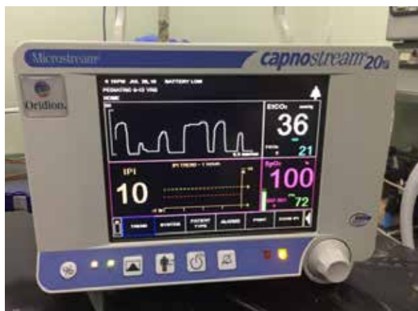
Fig 1: The Integrated Pulmonary Index monitor (Capnostream 20p; Medtronic, Inc., Minneapolis, MN, USA) demonstrating the respiratory score (A) calculated based on end-tidal carbon dioxide (B), pulse rate (C), peripheral oxygen saturation (D) and respiratory rate (E).
